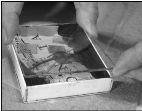
Since the glass is the same size as the back, it will sit on top of the box sides rather than fit inside the opening.
