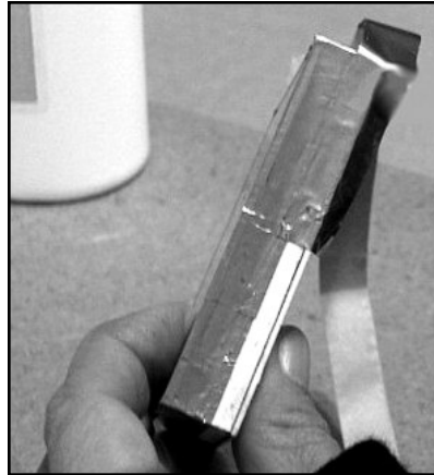
In this photo, the first piece of copper tape has already been applied to secure the glass to the box. Now I’m adding the second piece of tape along the bottom edge. You also can see how the box sides sit on top of the back piece.
